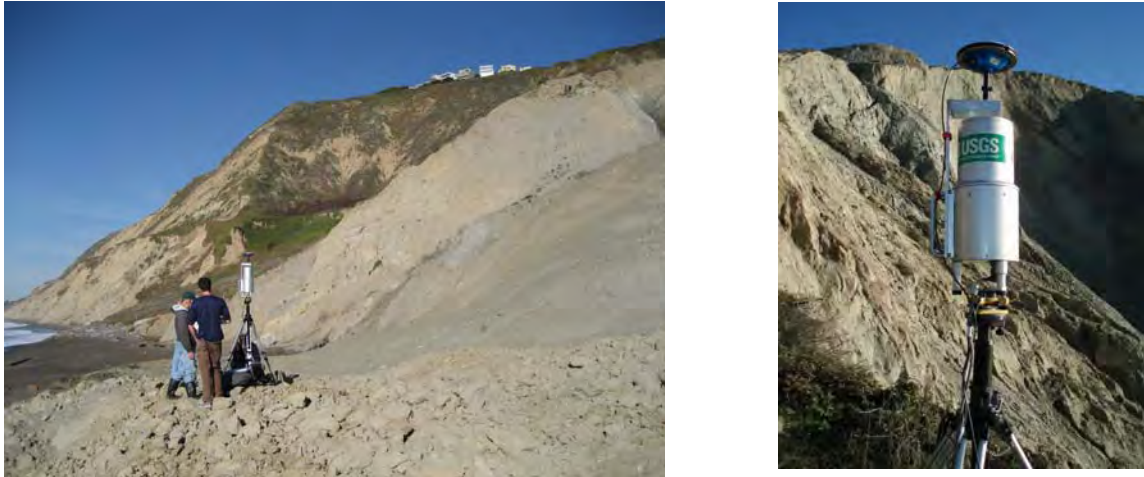
Figure 6. The USGS Coastal and Marine Geology program's terrestrial LIDAR unit at the Northridge Bluff Landslide. Close-up shows laser and GPS antenna used for georeferencing instrument location.
