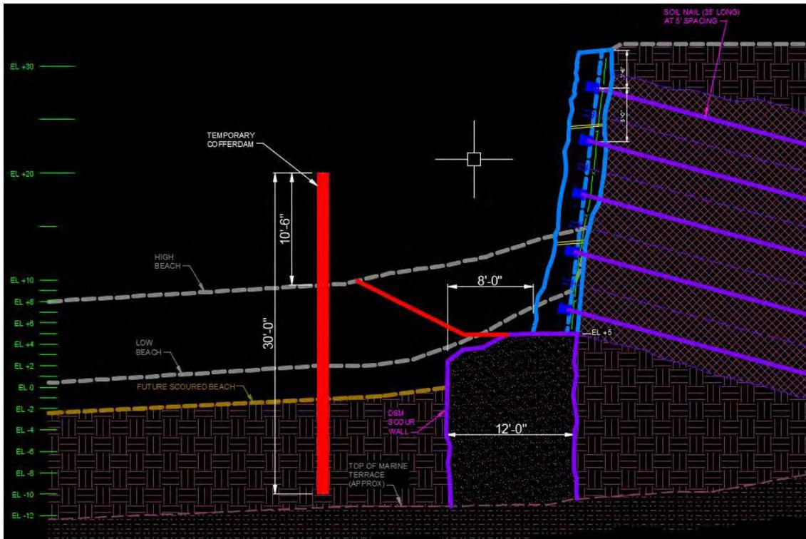
Figure 6. Deep Soil Mixed Wall alternative.
