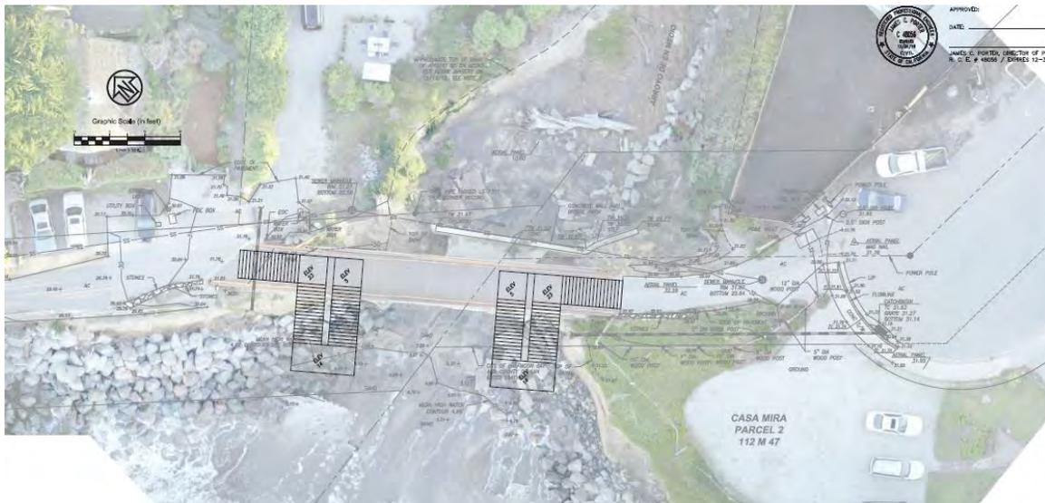
**Figure 5.** Seasonal access alternative with staircases on northern and southern bluff walls leading into Arroyo de en Medio.
