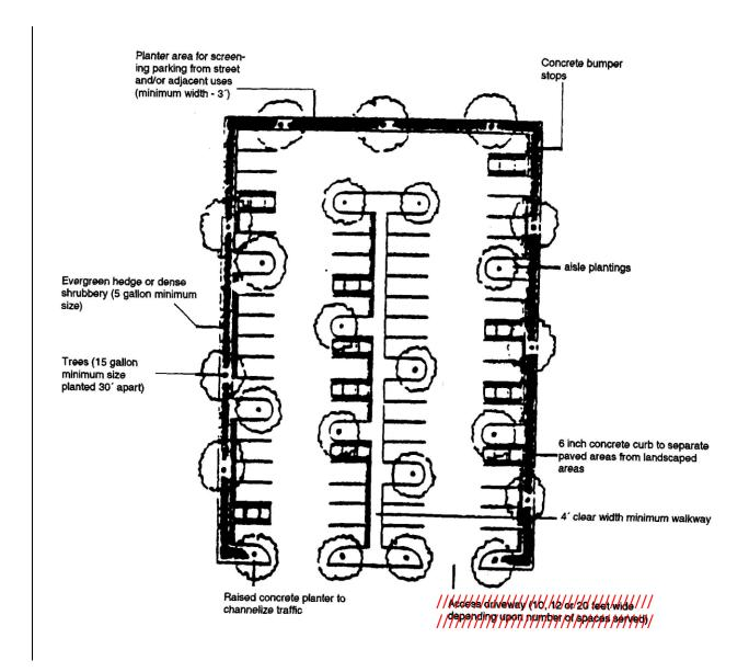
This diagram appears at the end of Chapter 24.12. The lower right-most caption contains confusing and inaccurate details and is proposed for deletion. The remaining illustrations as well as the proposed text in Section 24.12.280.3(b) include correct information making this notation unnecessary.
