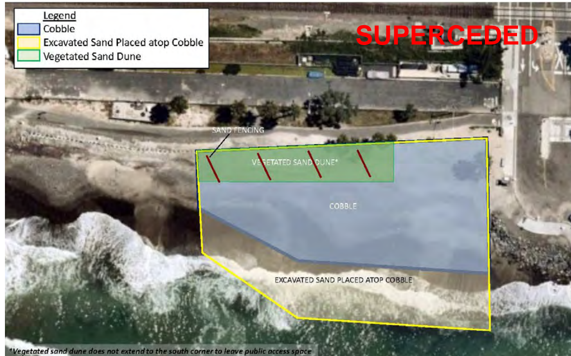
FIGURE A-9. NORTH REACH – BURIED COBBLE BERM AND VEGETATED DUNE CONCEPT – PLAN VIEW (SUPERCEDED)
