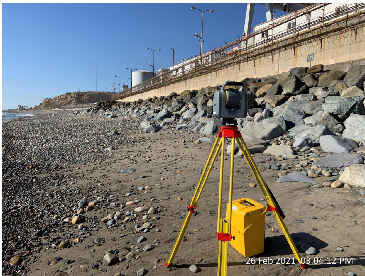
Figure 4-8. Photo of Trimble SX10 scanning total station used by Coastal Environments for SONGS topographic surveys.
