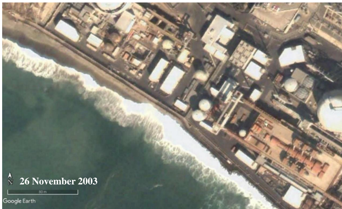
Photo D-3. Photograph showing waves attacking the revetment and the presence of a sand beach at the northern end of SONGS (26 November 2003).
