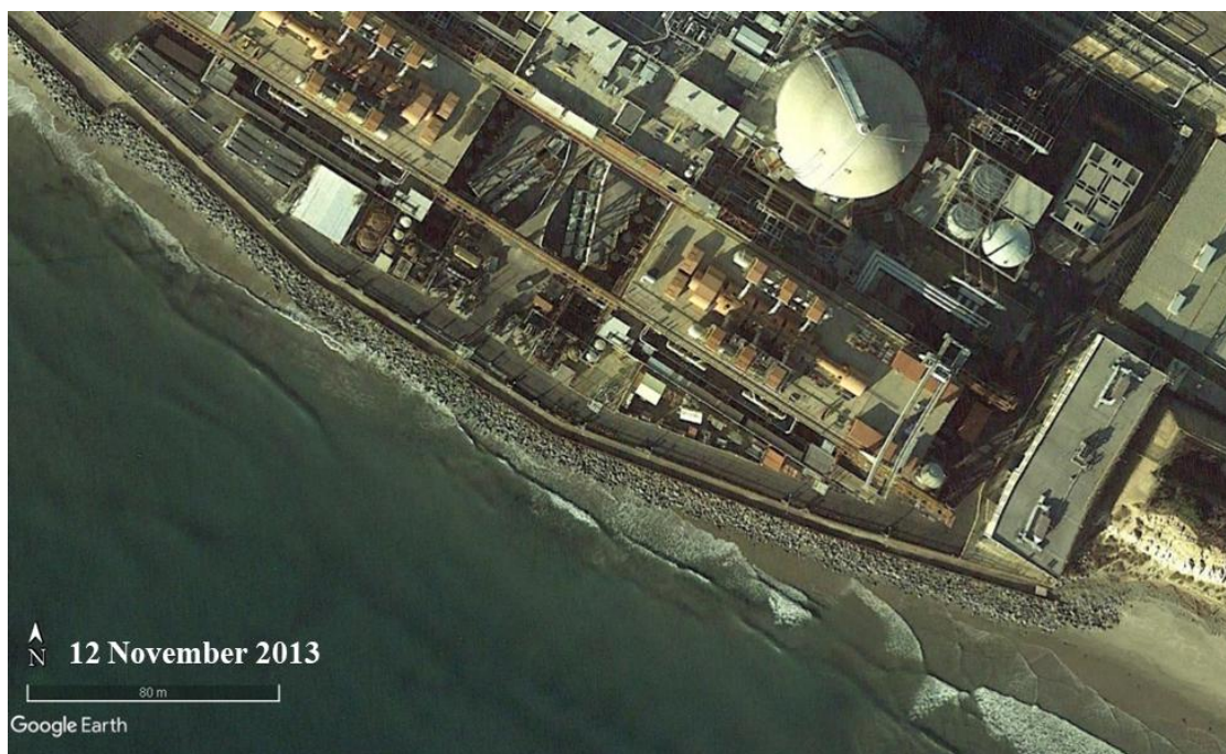
Photo D-12. Photograph showing waves attacking SONGS revetment and refracting towards south at the southern end of SONGS (12 November 2013).
