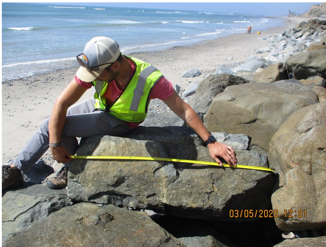
Figure 4-5. Measurement of long axis (length) of riprap rock.
