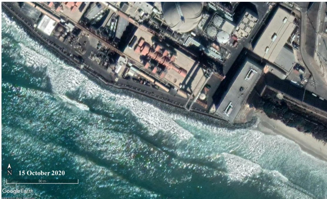
Photo D-20. Photograph showing waves attacking SONGS revetment and refracting towards south at the southern end of SONGS (15 October 2020).
