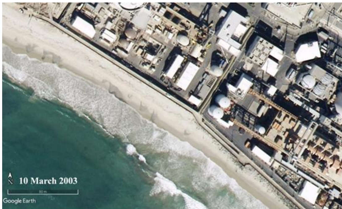
Photo D-1. Photograph showing revetment covered by sand and fronted by a wide beach at the northern end of SONGS (10 March 2003).
