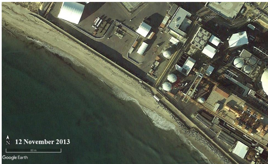
Photo D-11. Photograph showing revetment covered by sand and fronted by a wide beach at the northern end of SONGS (12 November 2013).
