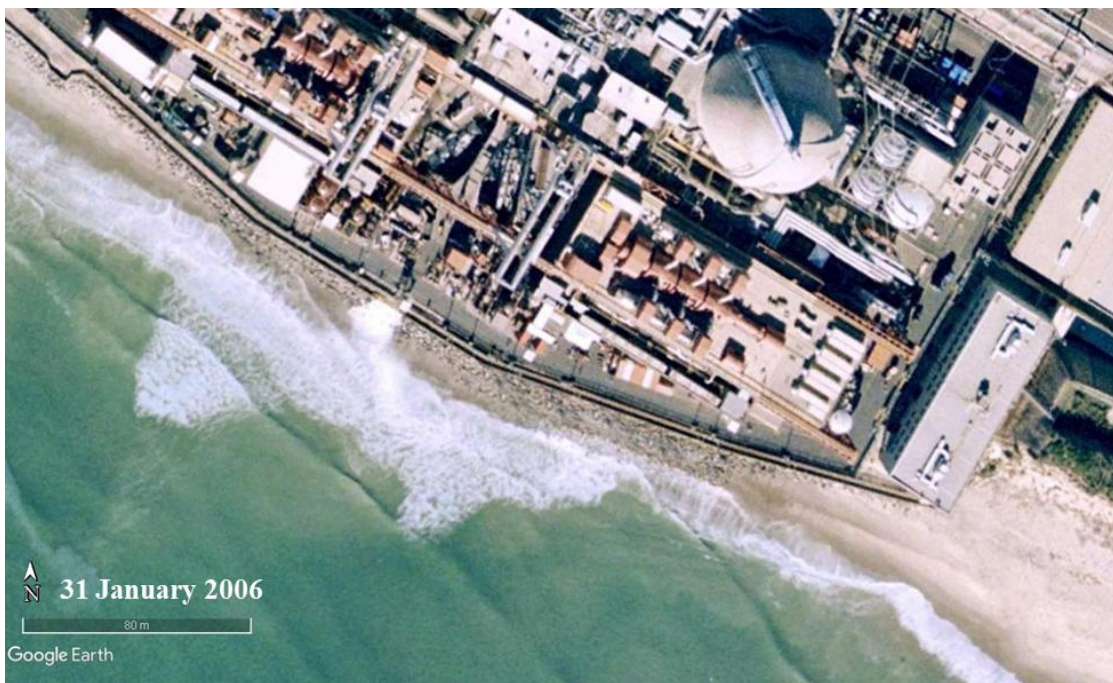
Photo D-8. Photograph showing waves from north swell attacking SONGS revetment and refracting towards south at the southern end of SONGS (31 January 2006).
