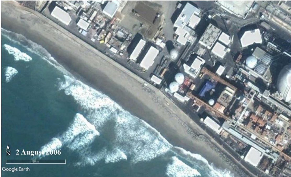
Photo D-5. Photograph showing revetment covered by sand and fronted by a wide beach at the northern end of SONGS (2 August 2006).
