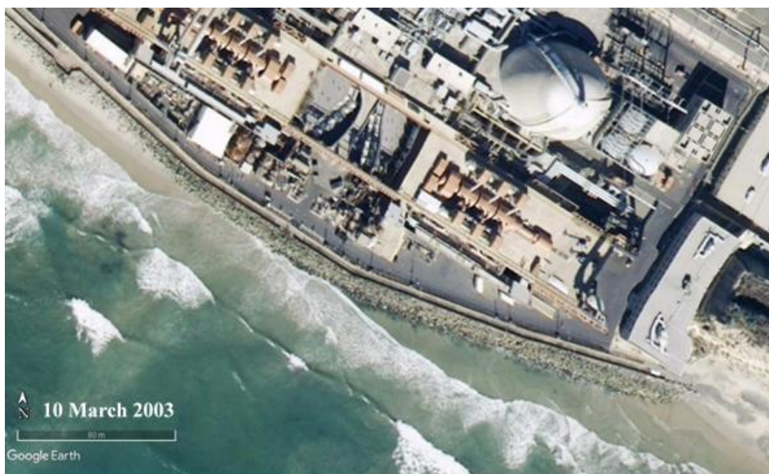
Photo D-2. Photograph showing waves from north swell attacking SONGS revetment at the southern end of SONGS (10 March 2003).
