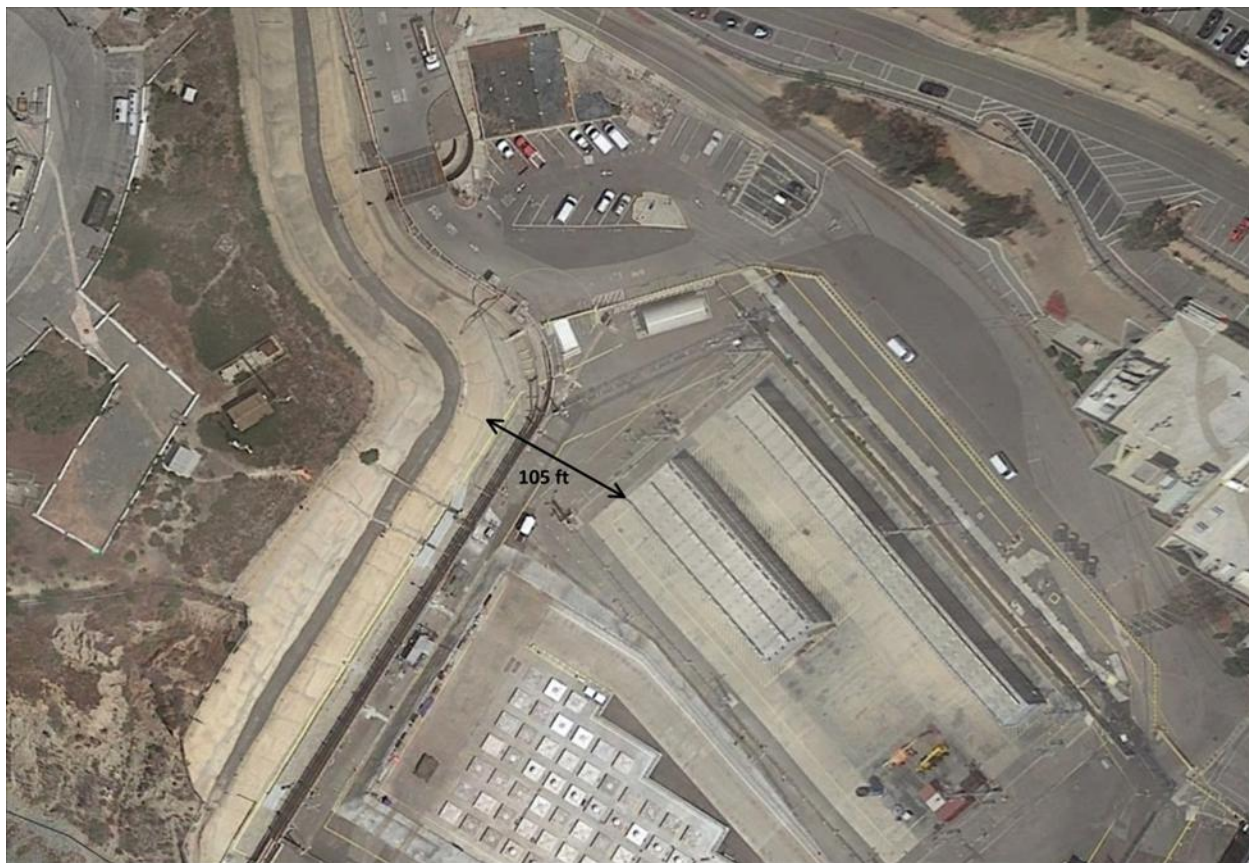
Figure 2-12. Plan view of Holtec (west, lower) and NUHOMS (east, upper) ISFSIs. Minimum distance between the north and east bluffs is 105 ft.
