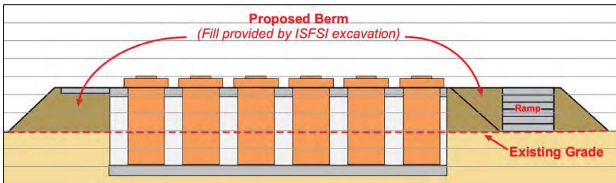
Figure 1. Cross section illustration of the concrete pads and storage modules. The space between the cylindrical storage modules is filled with concrete.
