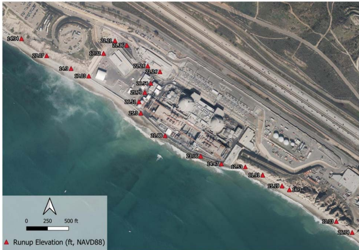
Figure 6. SONGS aerial view showing tsunami run-up data, taken from https://ASCE7tsunami.online .
