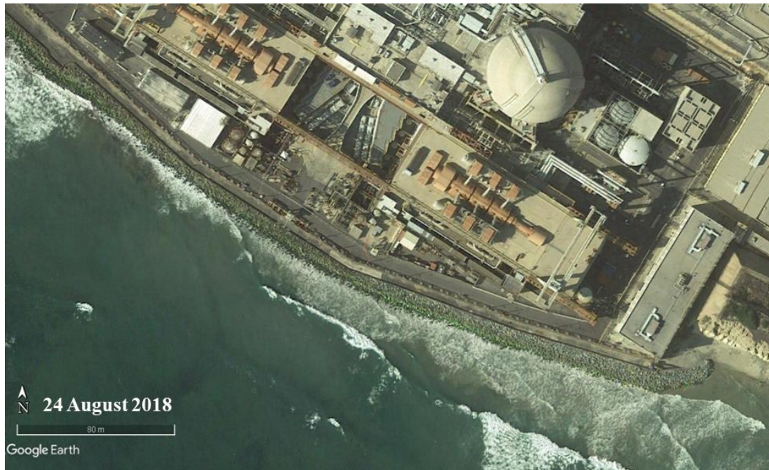
Photo D-18. Photograph showing waves from north swell attacking SONGS revetment and refracting towards south at the southern end of SONGS (24 August 2018).
