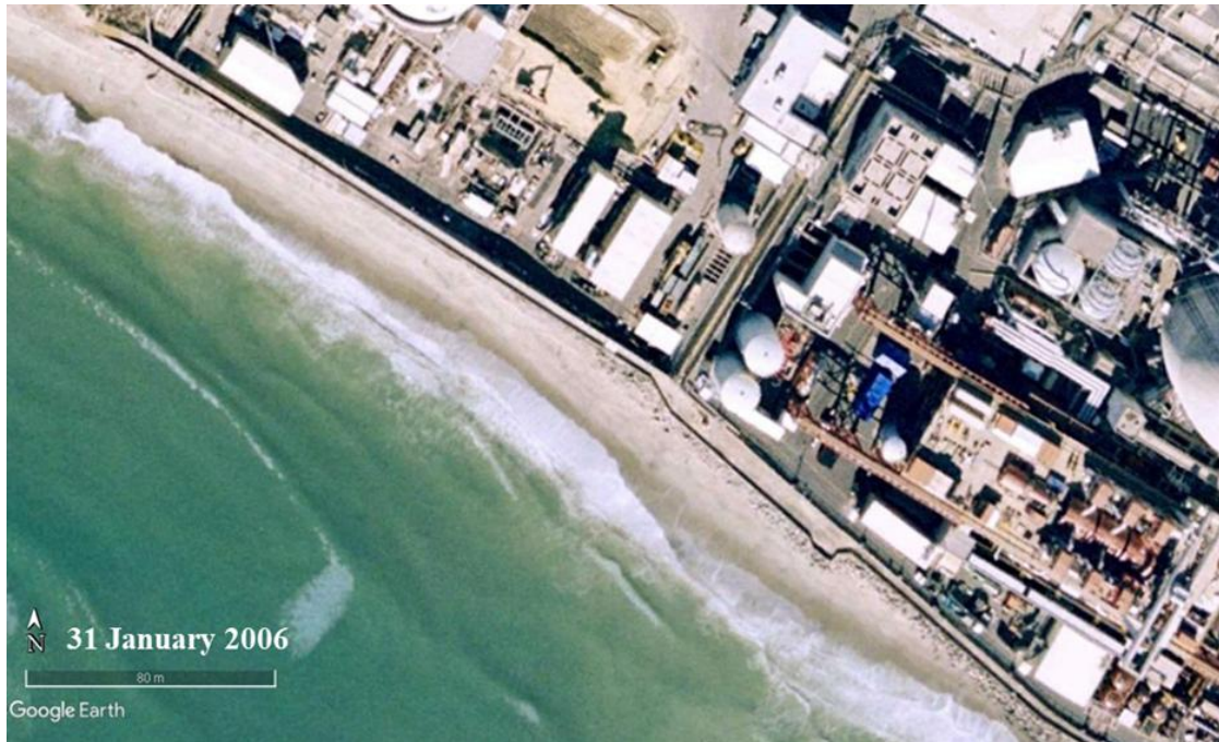
Photo D-7. Photograph showing revetment covered by sand and fronted by a wide beach at the northern end of SONGS (31 January 2006).
