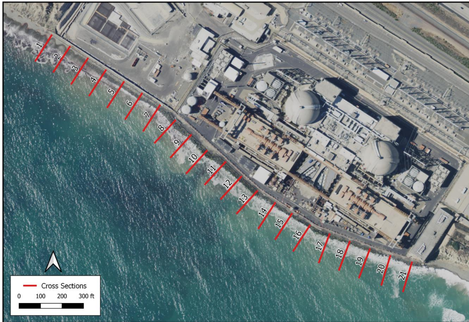
Figure B-1. Locations of 21 transects along the revetment, spaced 100 ft apart.
