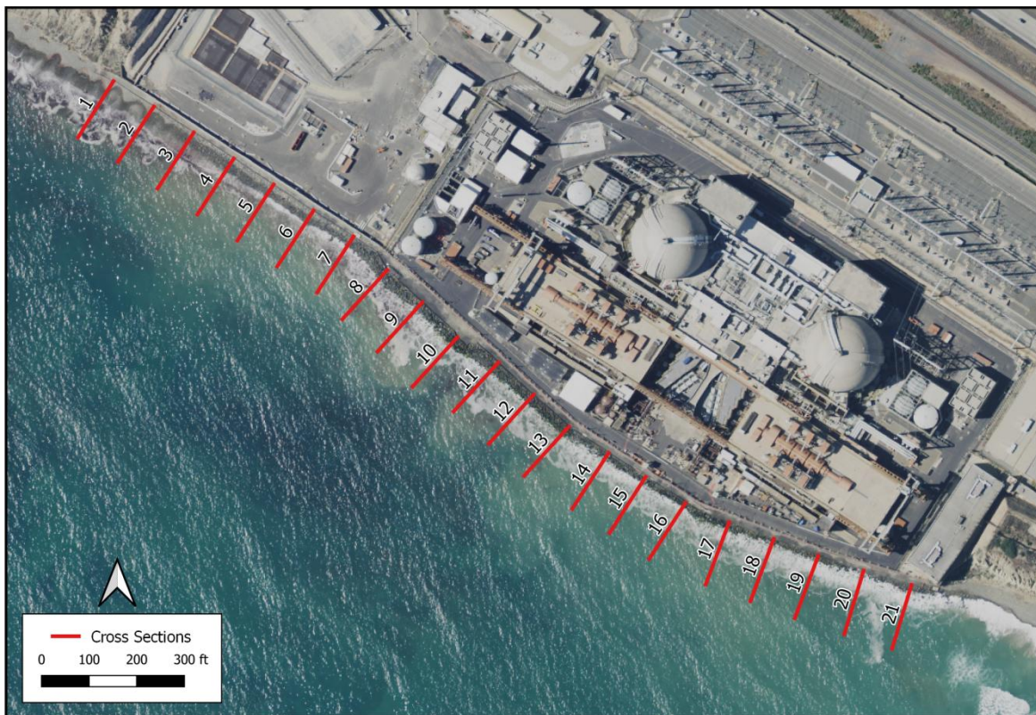
Figure 4-9. Location of 21 transects along the revetment, spaced 100 ft apart.
