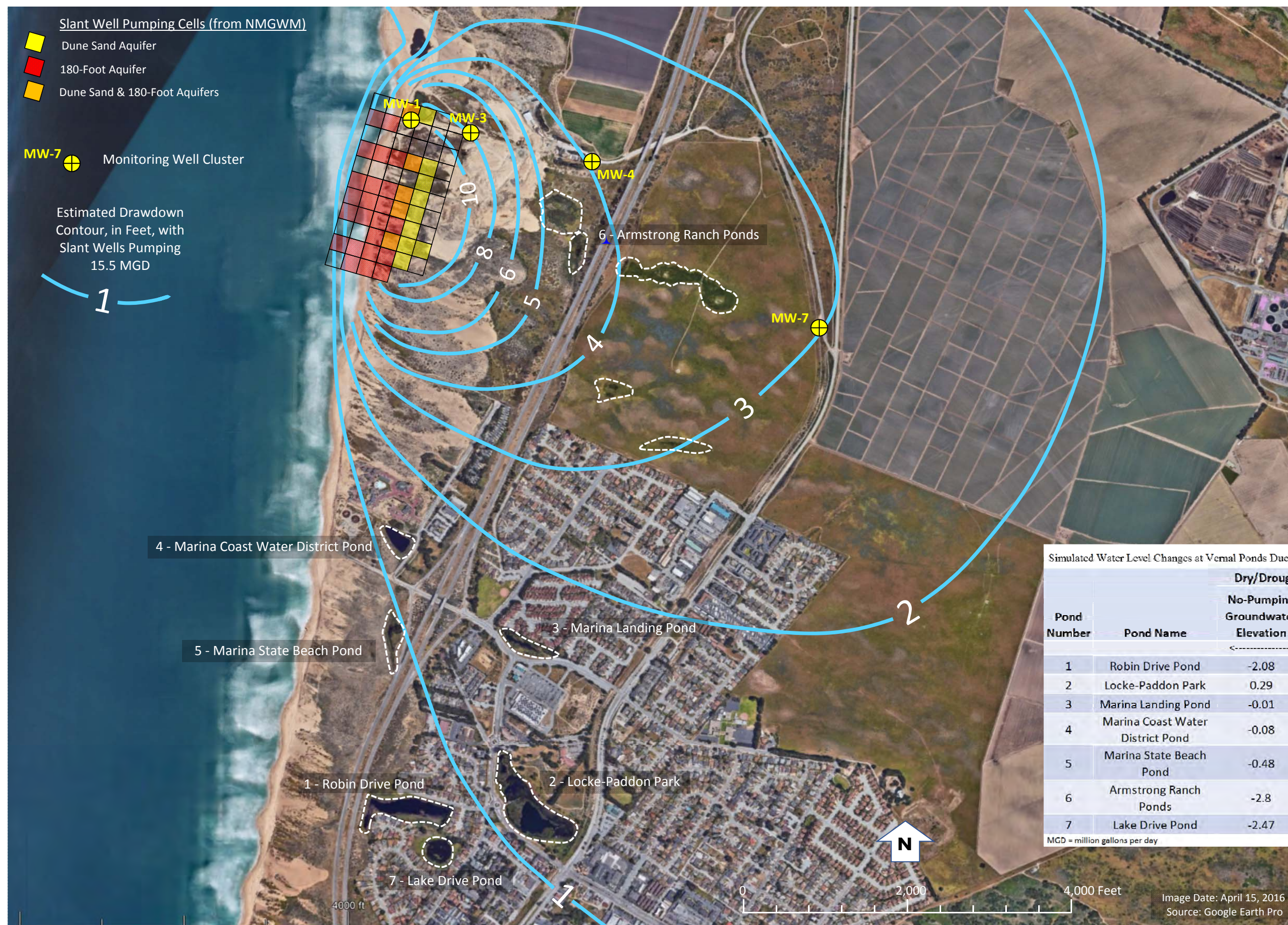
Figure 1. Location of Vernal Ponds Relative to Slant Wells, and Estimated Drawdown, Slant Wells Pumping 15.5 Million Gallons Per Day (MGD)
