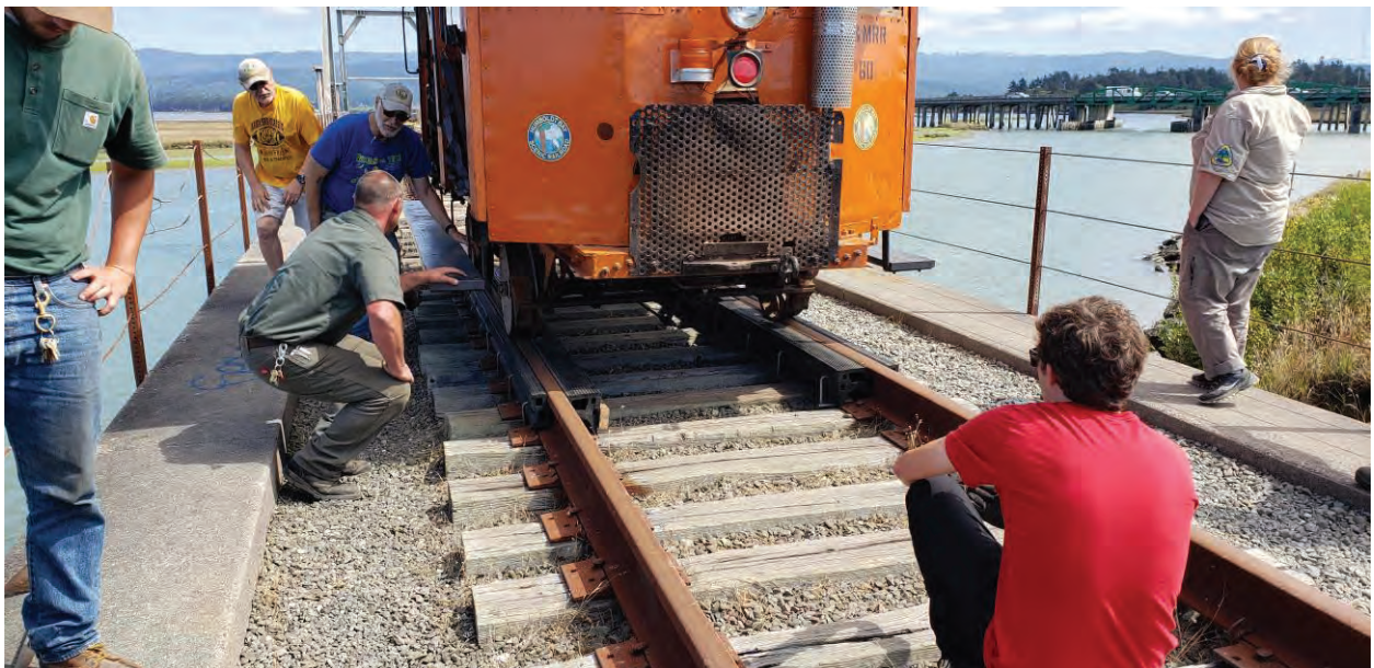
Photo 4 (September 6, 2019): Test of flangeway filler products on Eureka Slough Bridge (Segment 2).
