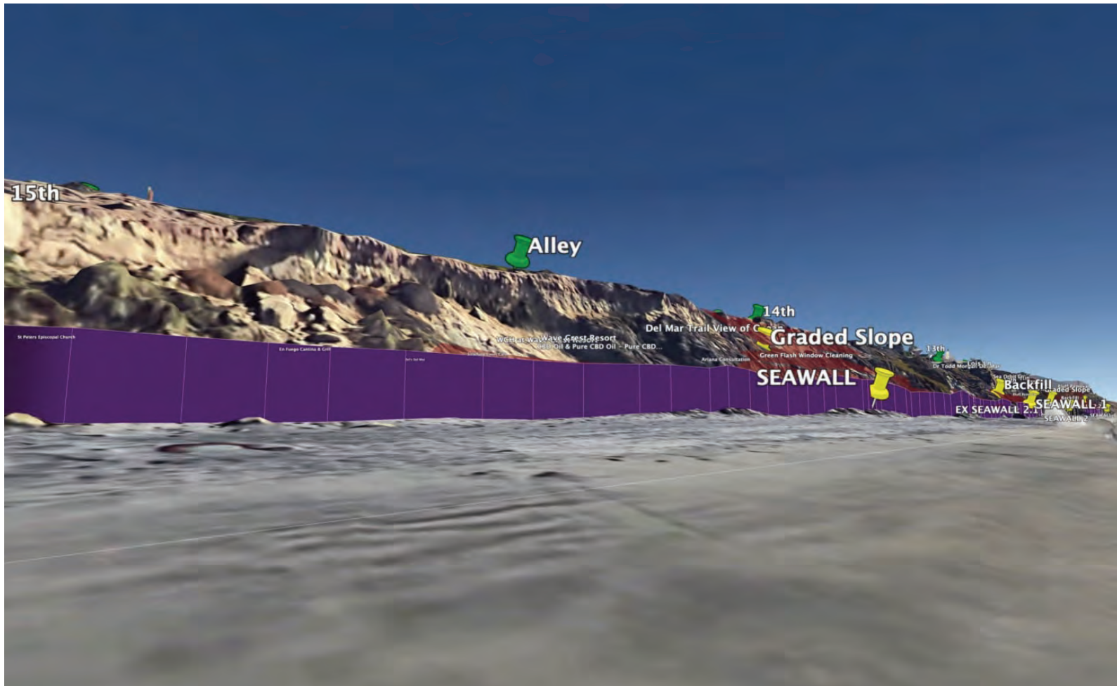
Figure 7. Del Mar Bluff Engineering, Seawall at Beach Level below 15 th St to 11 th St Continuous seawall (purple) along the toe of the bluffs, 8-foot height. Red shaded areas show graded slopes. Yellow pins mark specific engineered structures, including seawalls, back-fill, and graded slopes. Bluff top, 61-65 feet above sea level.
