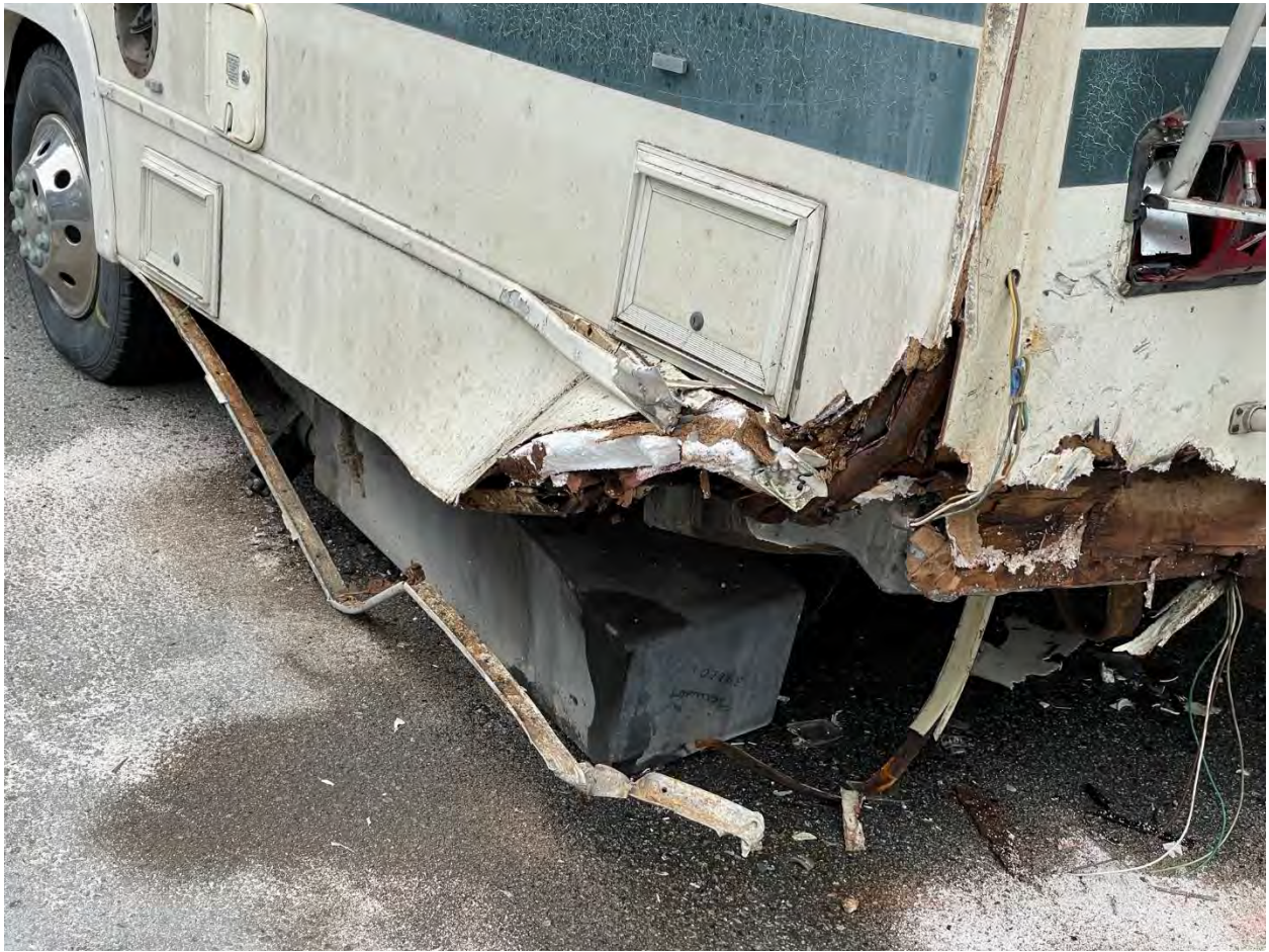
Figure 8 - The blackwater tank from the vehicle was damaged and hangs from the bottom on the ground. It is seen leaking fluid into the street and the storm drain. This vehicle remained here for over a week despite calls to the city to have it removed.
