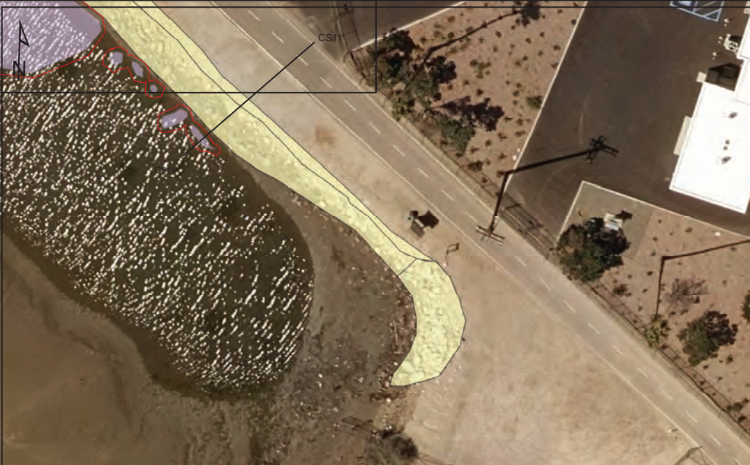
Broken concrete blocks to be removed from slope and replaced with clean rip rap.
