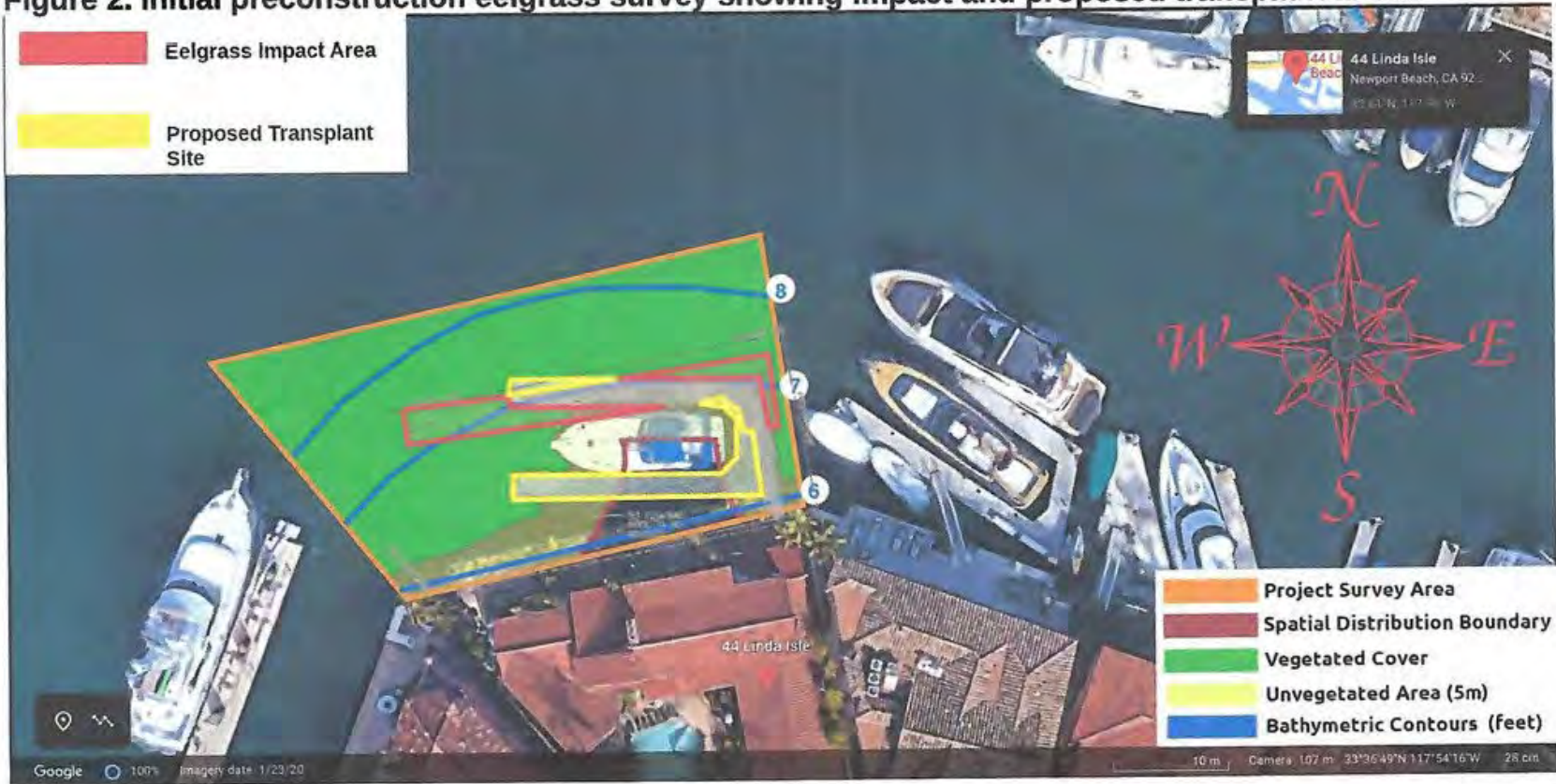
Figure 2. Initial preconstruction eelgrass survey showing impact and proposed transplant areas.
