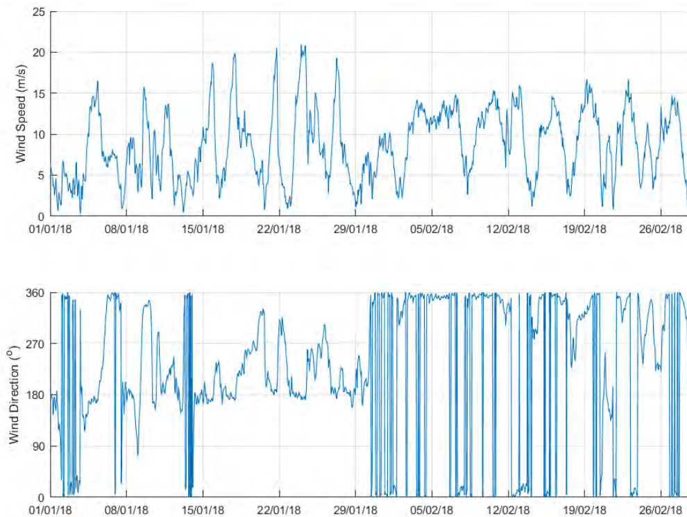
Figure 19 CFSv2 simulated wind data at the North Spit from January to March 2018 (water level verification period).
