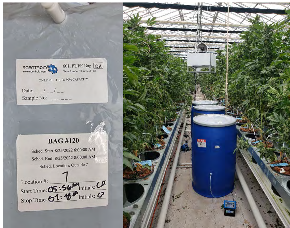
Figure 4. Sampled 60L PTFE Bag and ≈35 Gallon Lung Sampler with GilAir Pump
