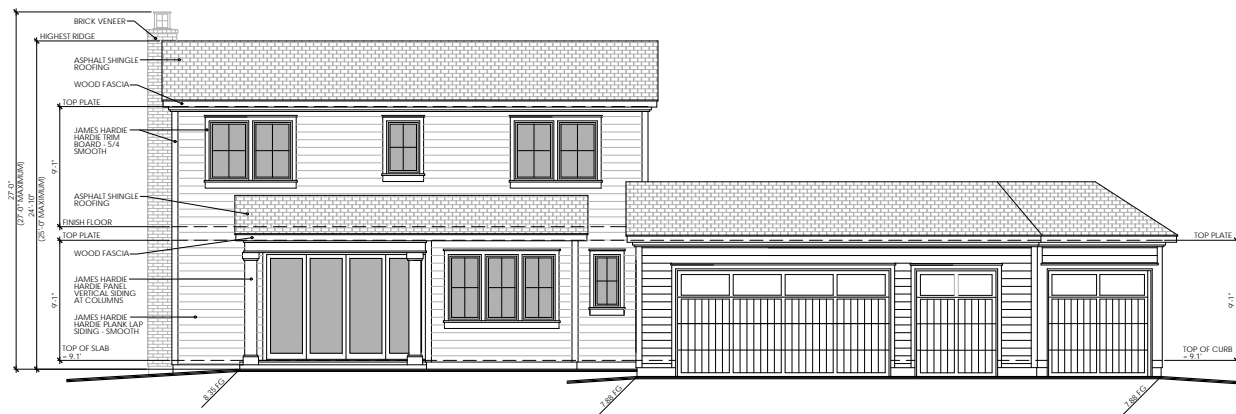
EAST ELEVATION SCALE : 1/4"=1'-0"
