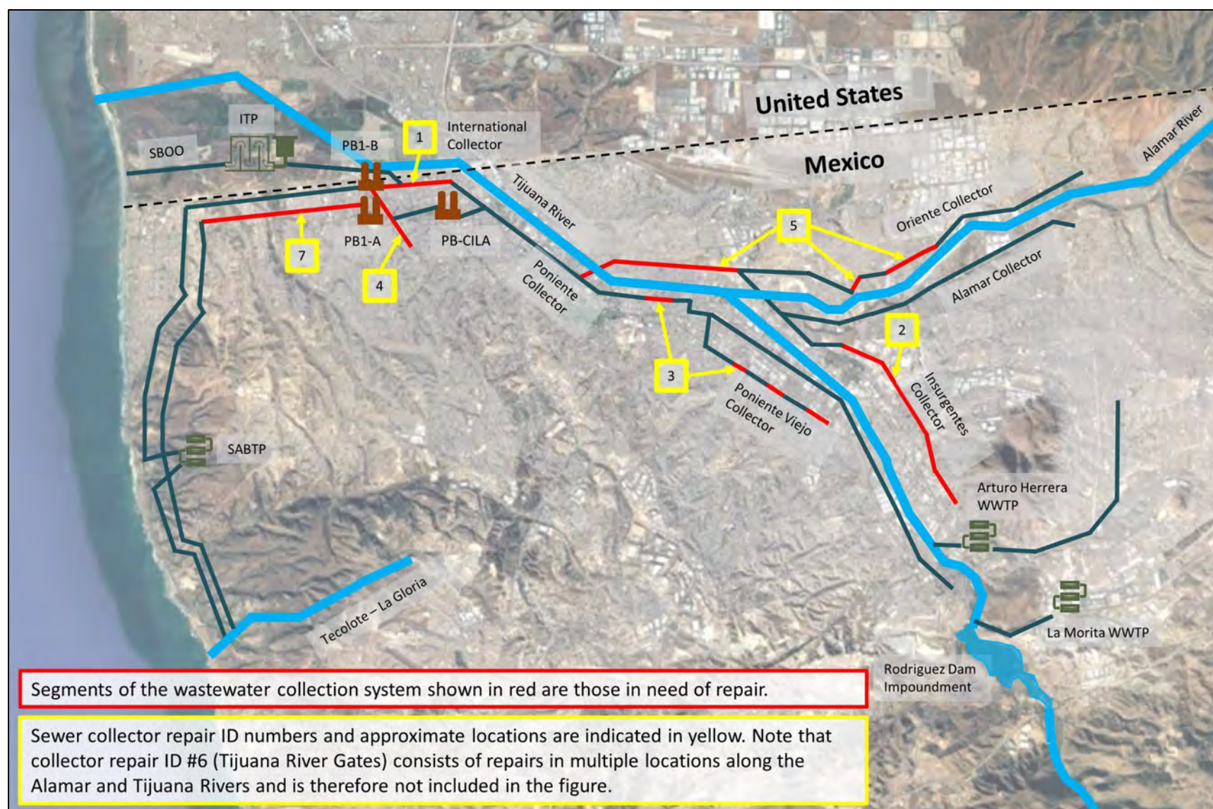
Figure 2-7. Project C (Tijuana Sewer Repairs) – Schematic of Tijuana Sewer Collectors for Rehabilitation or Replacement
