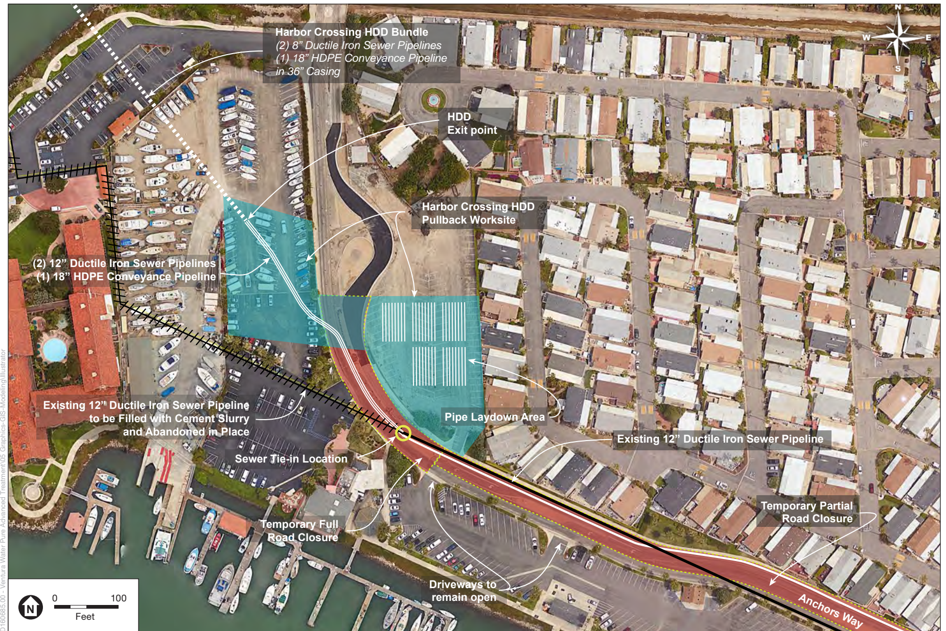
Figure 5e Harbor Crossing HDD Pullback Worksite
