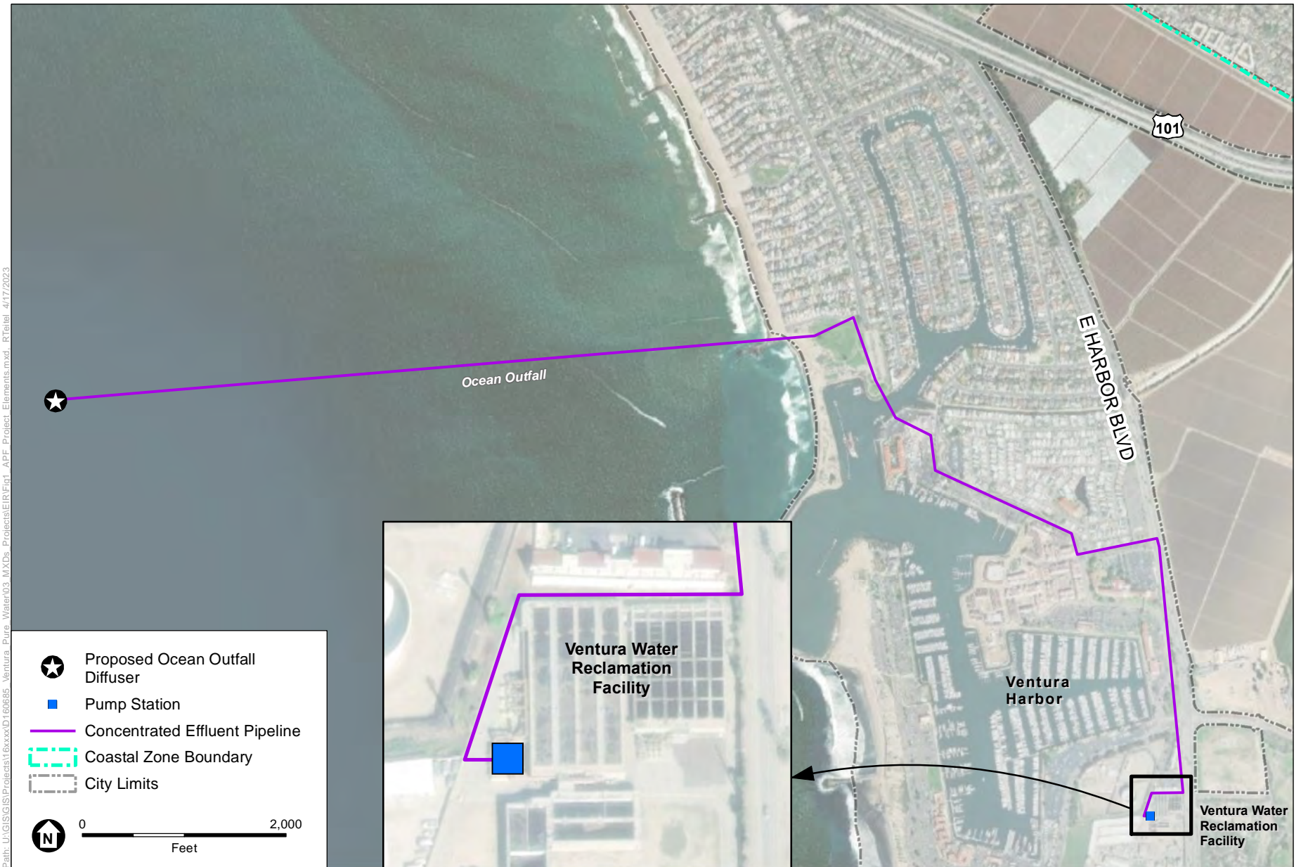
Figure 1 Ventura Water Pure Ocean Outfall Project Elements
