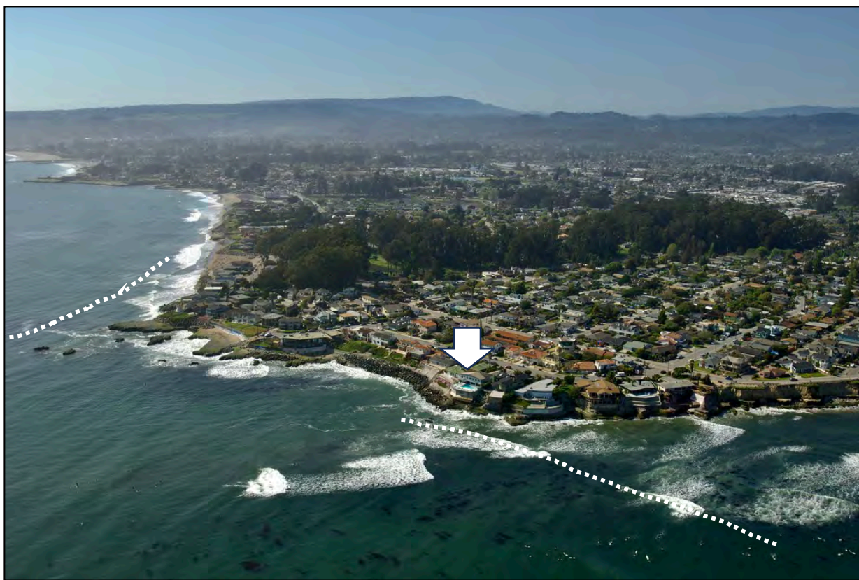
Figure 3. Wave refraction is what makes surfing optimal at Pleasure Point. The angle at which the waves approach the shoreline changes by about 90° as the waves bend around Soquel and Pleasure Points. Note where the surfers are concentrated compared to the locations of the properties on Pleasure Point Drive (arrow).
