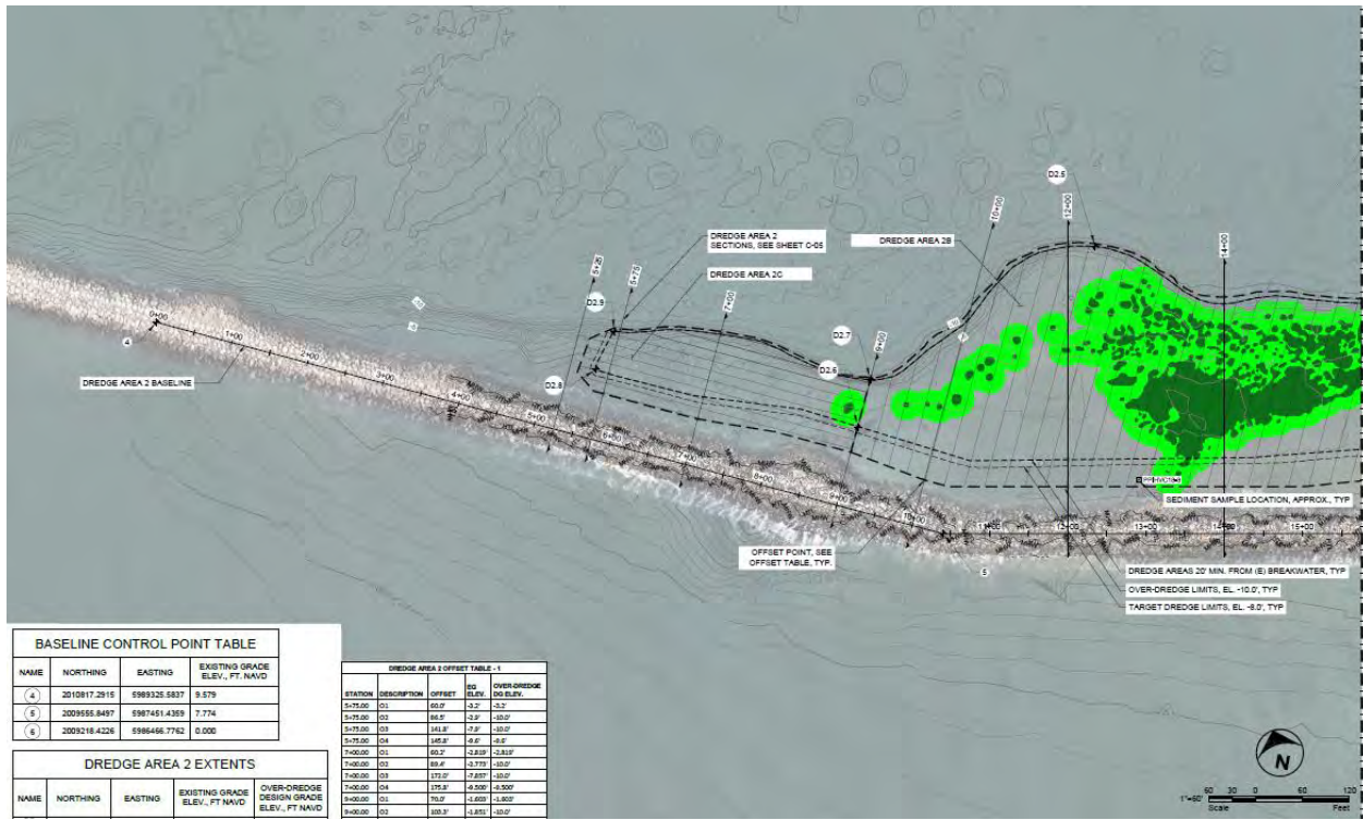
Figure 3. East basin dredge area plan – 2A.
