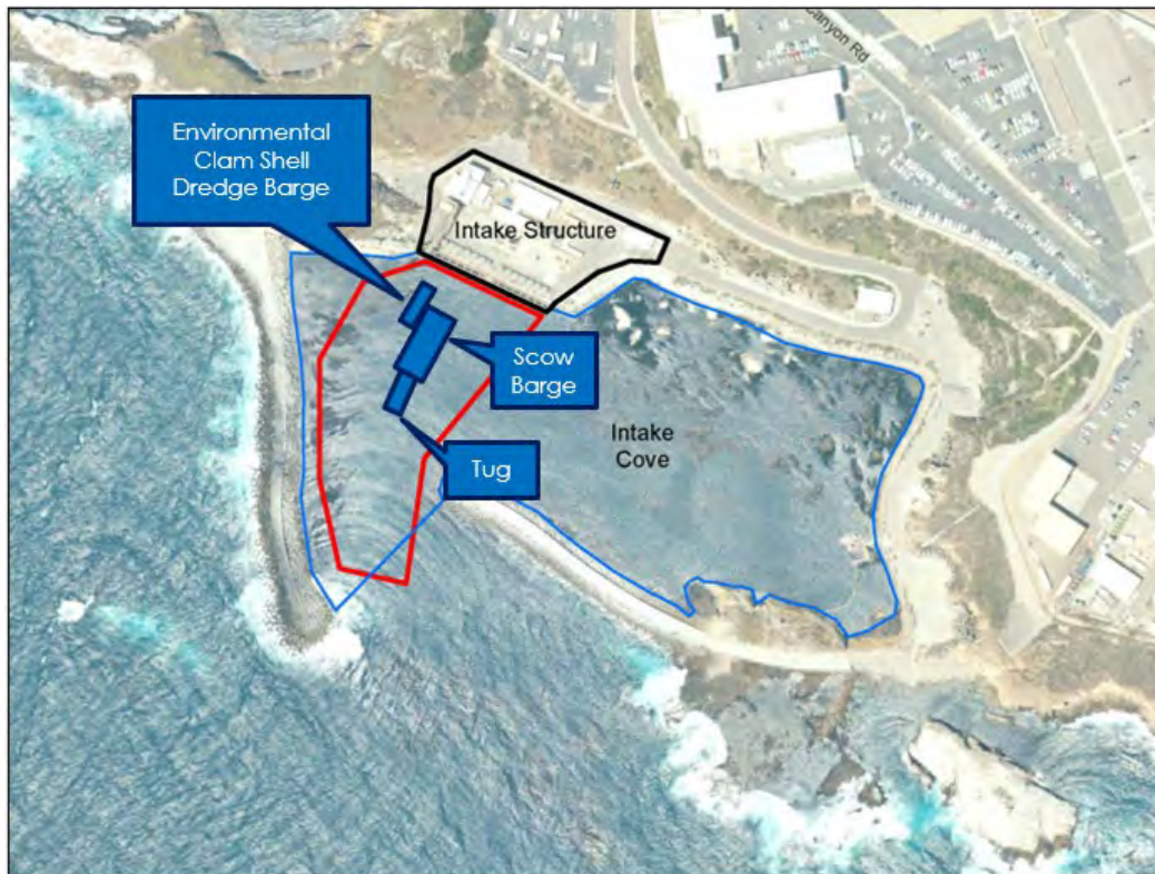
Exhibit B: Conceptual Clamshell Dredge Layout (Contingent Approach)
