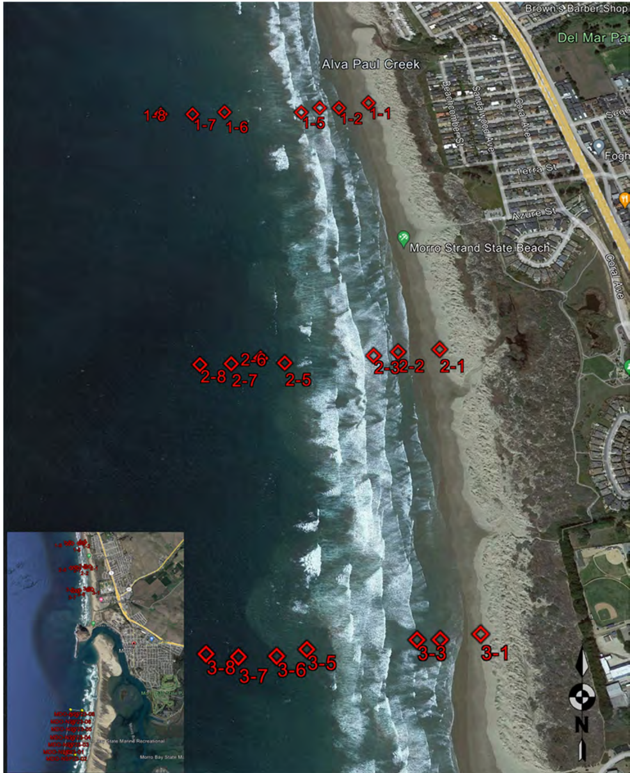
Figure 13. Approximate Locations of the Beach Sampling Transects at the Alternate Placement Area at Morro Strand State Beach (Note: Due to high surf and safety concerns, grab samples from transects at the -6 feet MLLW elevation were unable to be collected)
