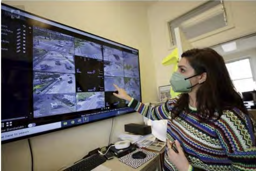
Monterey Engineering Assistant Marissa Garcia monitors the city's intersections from her office at City Hall using an artificial intelligence software program called SCOOT. It's connected to traffic lights that adjusts their timing in real time.
