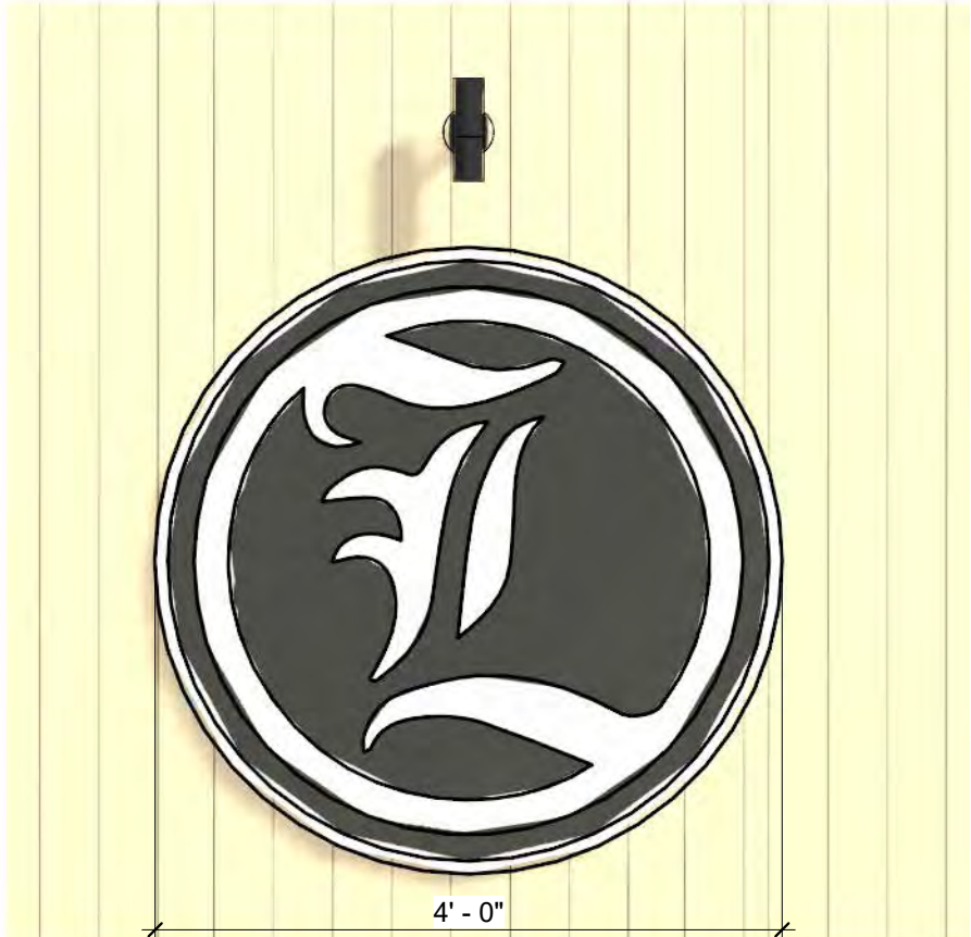
2 WALL SIGN (LOGO SOUTH) 3/4" = 1'-0" * SIGN TO BE METAL EXTERIOR ILLUMINATED. ATTACH PER MANUFACTURER SPECIFICATIONS.
