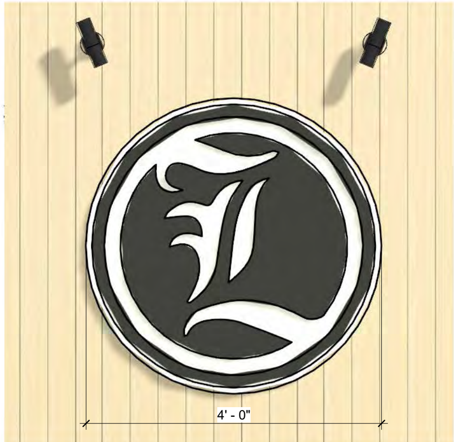
3 WALL SIGN (LOGO EAST) 3/4" = 1'-0" * SIGN TO BE METAL EXTERIOR ILLUMINATED. ATTACH PER MANUFACTURER SPECIFICATIONS. * PRIMARY FAÇADE SIGN
