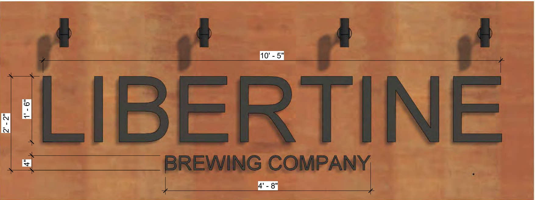
1 WALL SIGN (LETTERS MAIN) 3/4" = 1'-0" * SIGN TO BE METAL EXTERIOR ILLUMINATED. ATTACH PER MANUFACTURER SPECIFICATIONS.
