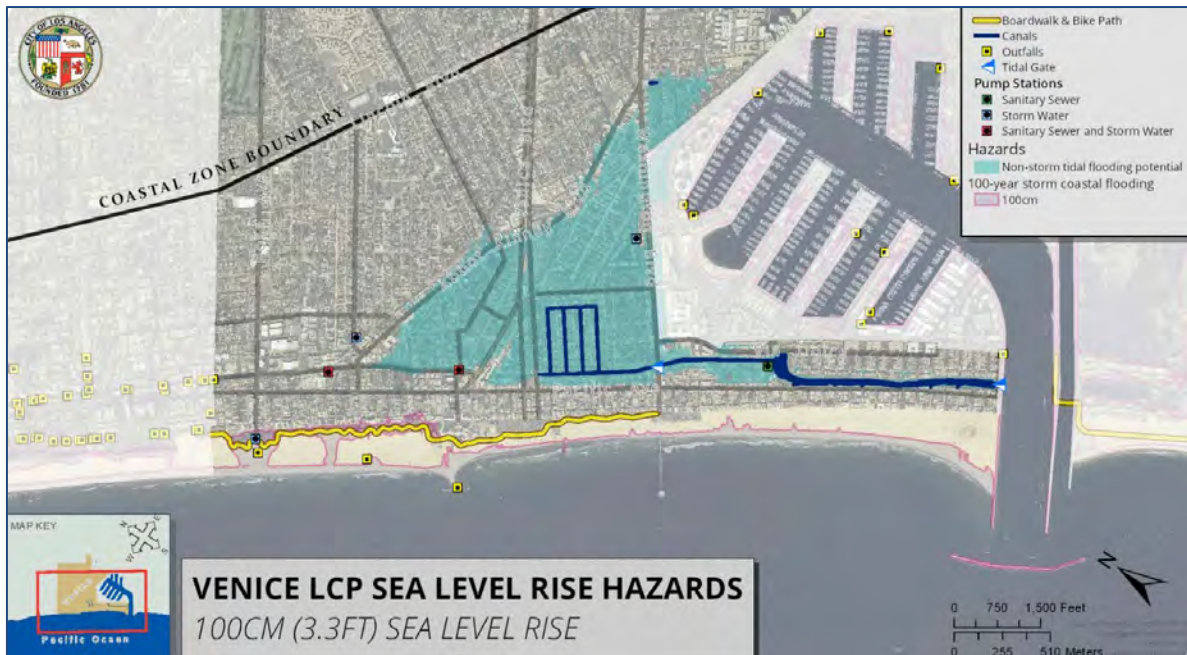
Figure 13. Example of analysis of SLR impacts. Hazards predicted from the CoSMoS mapping of 3.3 feet (100 cm) of sea level rise in Venice, CA. (Source: Venice Sea Level Rise Vulnerability Assessment 2018 ).
