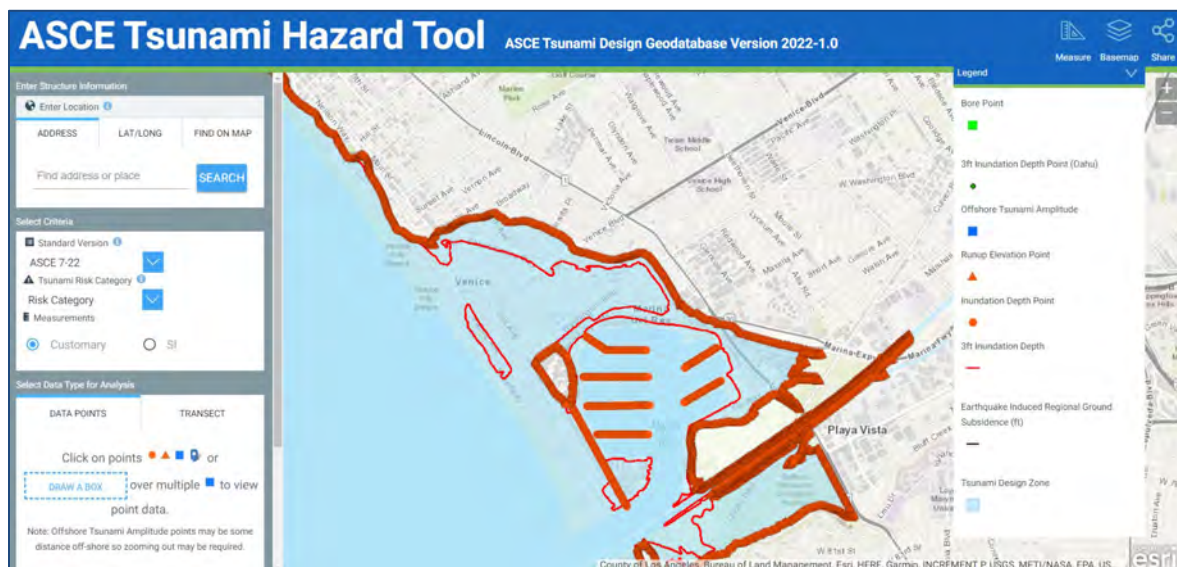
Figure B-10. Screenshot of ASCE Tsunami Hazard Tool showing results for the Venice-Marina del Rey area for the 2,475-year probabilistic tsunami hazard analysis
