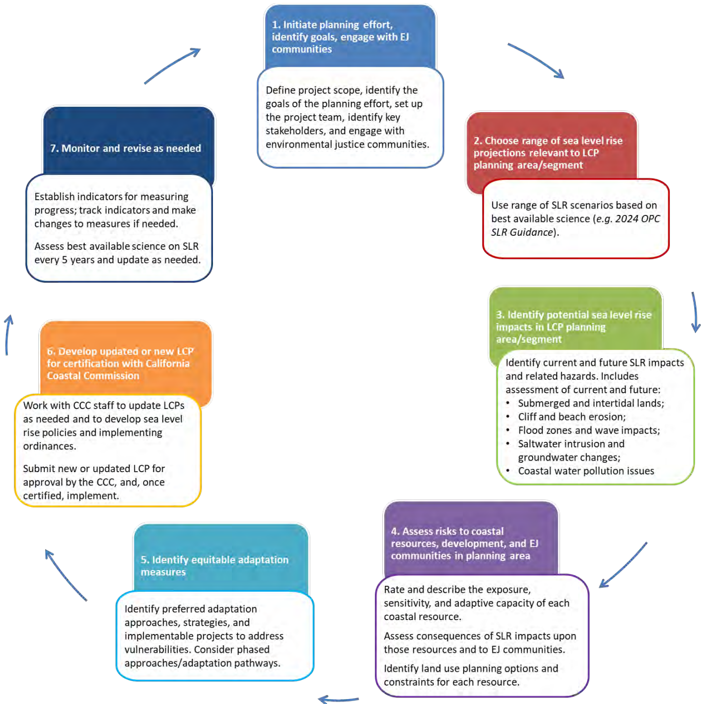
Figure 14. Flowchart for addressing sea level rise in Local Coastal Programs and other plans
