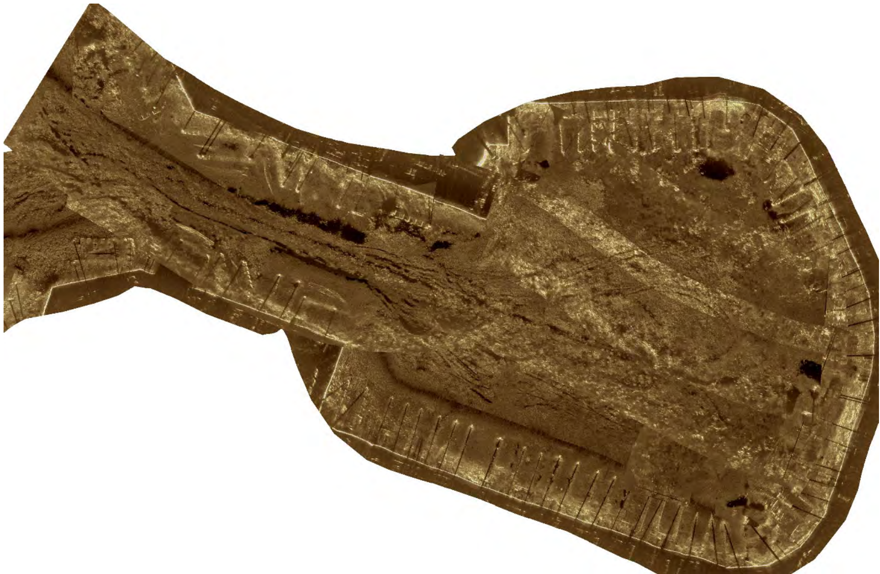
Figure 2. Interferometric sidescan sonar mosaic of Linda Isle Lagoon, March 2021
