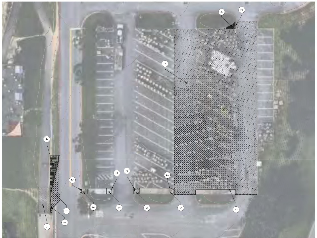
2 PARKING LOT DEMOLITION PLAN SCALE: 1" = 20'
