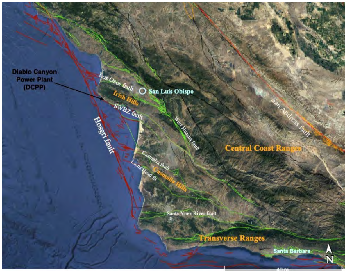
Fig. 2 Map of known Quaternary active faults near the Diablo Canyon Power Plant.
