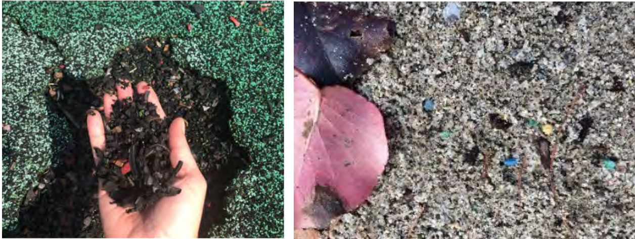
Left: Deteriorated top wear layer of PIP rubber playground exposing tire shreds underneath. Right: Synthetic rubber granules shed from a PIP rubber playground in sand near the playground. Photos courtesy of University of Massachusetts, Lowell Center for Sustainable Production. 55
