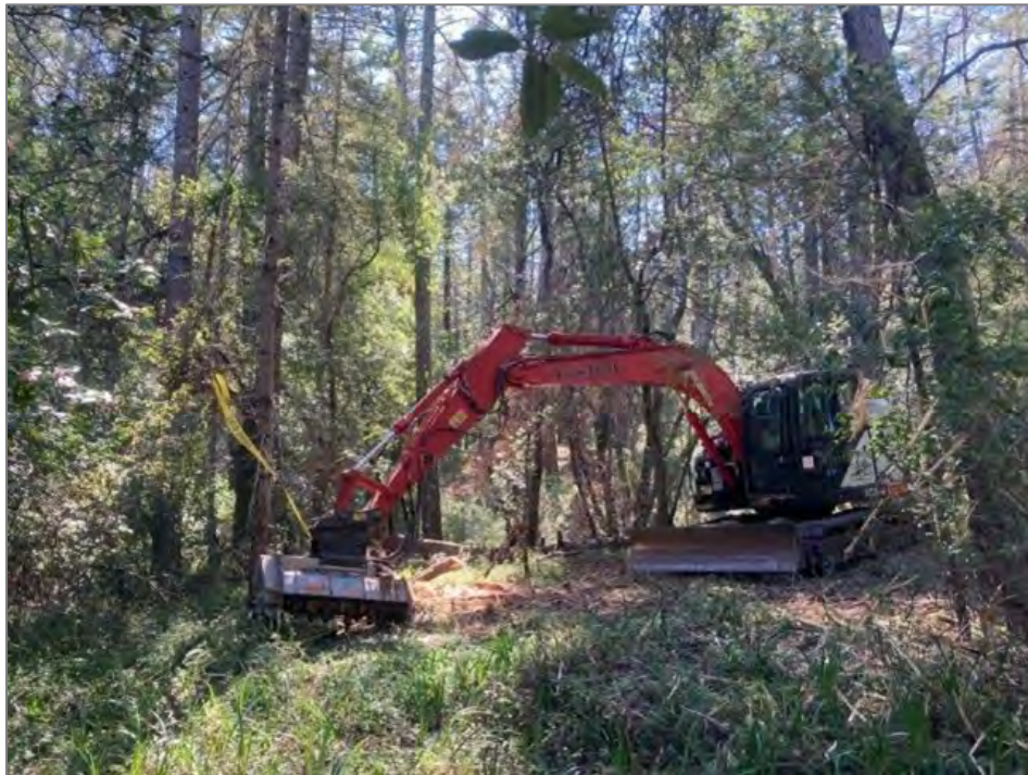
Figure 2-20 Example of Mechanized Equipment: Link-Belt 145 x 4 Excavator with Masticating Head Attachment
