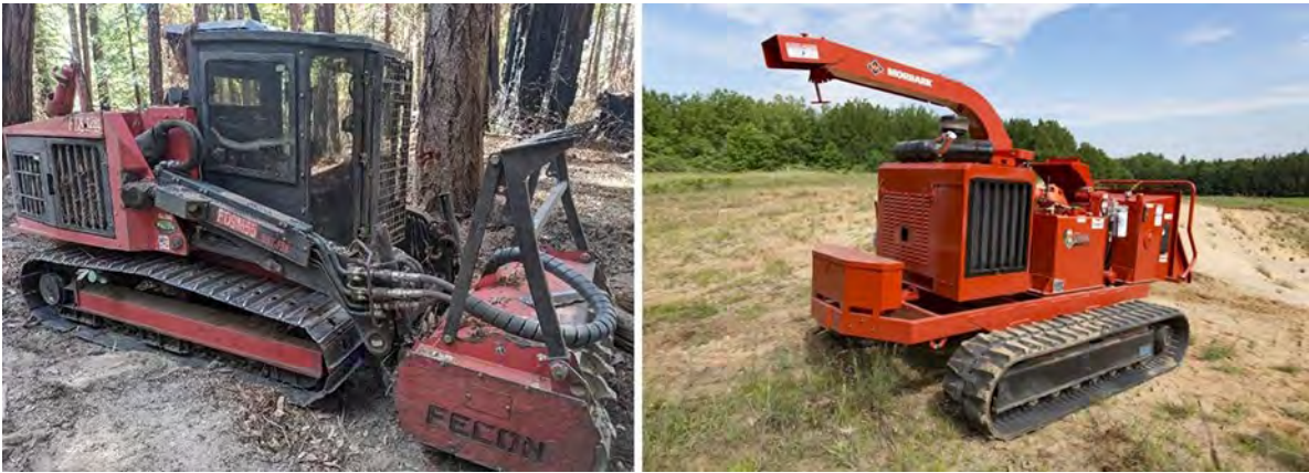
Figure 2-19 Examples of Mechanized Equipment: Fecon FTX 128 Series Compact Track Loader with Masticating Head Attachment (Left) and Morbark Beaver M15R Tracked Chipper (Right)
