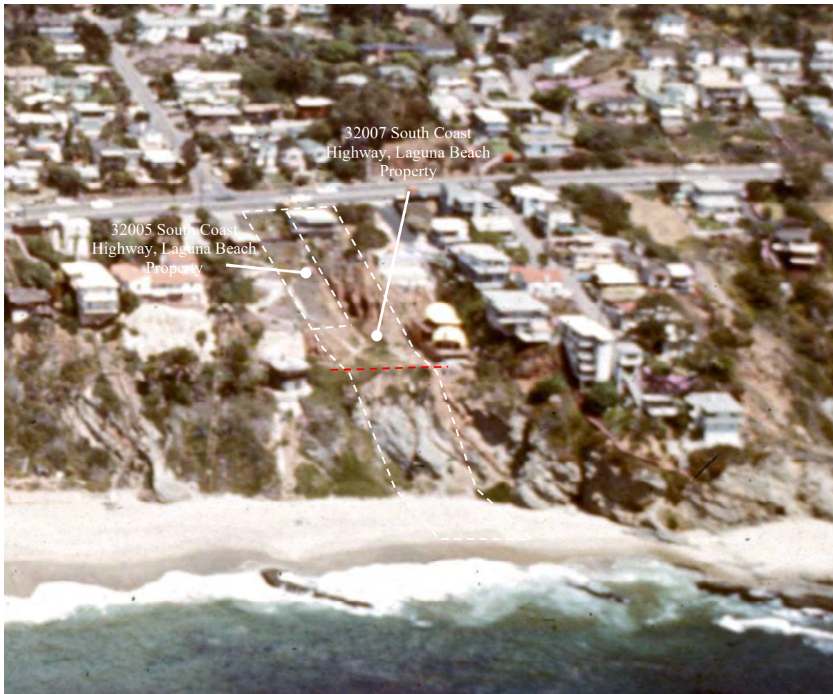
Photo 1: Close-up of a portion of California Coastal Records Project frame 7238102 dated 1972, showing the 32005 and 32007 properties prior to the 32007 residence construction. Approximate property lines depicted in white dash. Interpreted bluff edge depicted in red dash. The origin of the bench at elevation 89 feet appears to be the result of non-marine terrace retreat and gully erosion depositing onto a more resistant marine terrace, forming a level bench.
