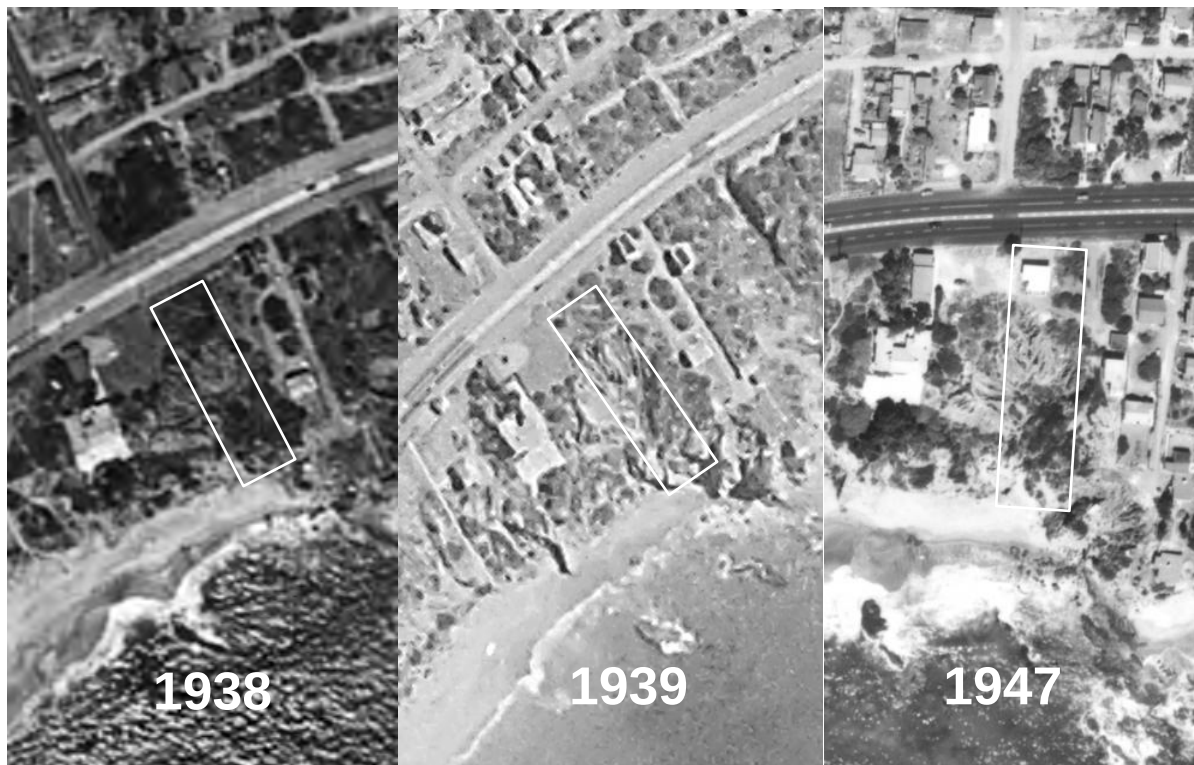
Figure 3: Aerial overview of property in 1938, 1939, and 1947, showing surface rilling of the terrestrial slope surface. No shoreline erosion or bluff edge is present above beachside cliff.
