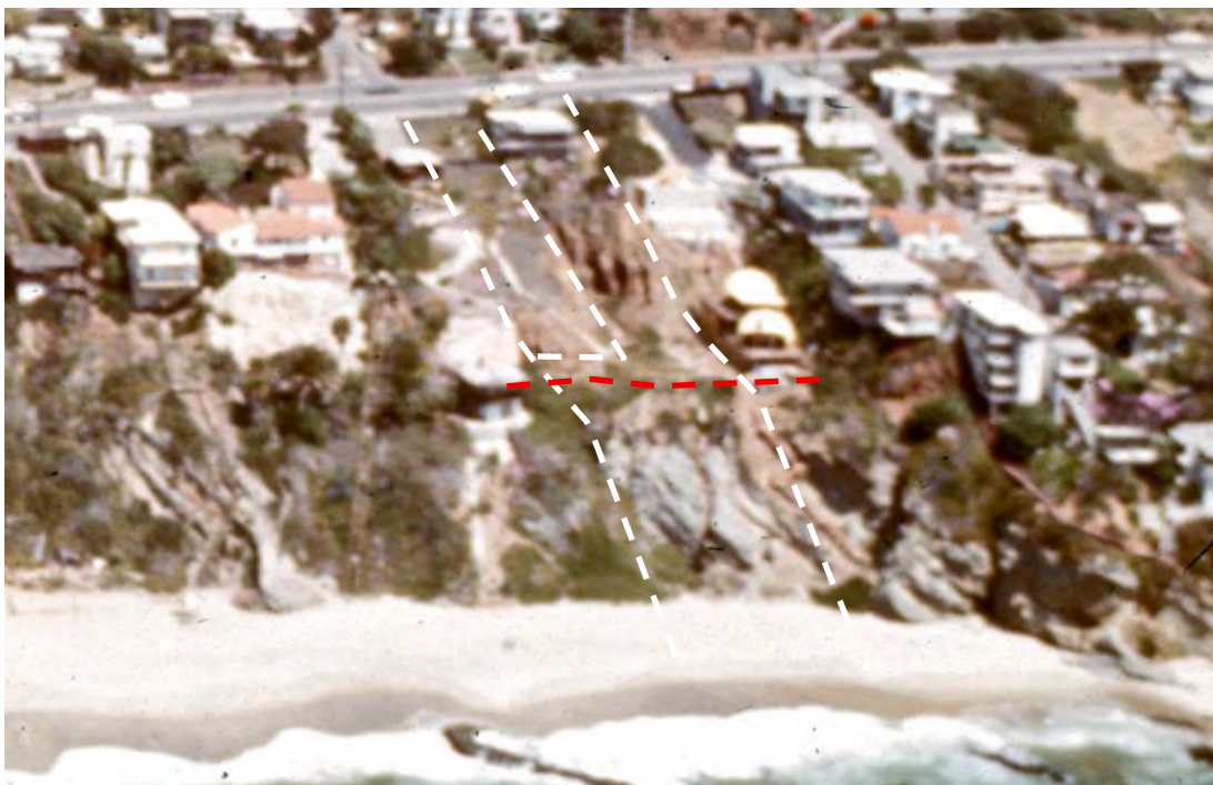
Figure 4: Close-up of a portion of California Coastal Records Project frame 7238102 dated 1972, showing the 32005 and 32007 properties prior to the 32007 residence construction. Approximate property lines depicted in white dash. Interpreted bluff edge depicted in red dash. The origin of the bench at elevation 89 feet appears to be
