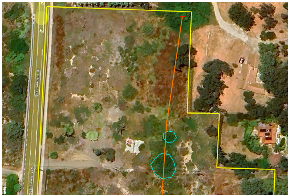
Exhibit 1. Aerial imagery dated June 29, 2023, showing in cyan the two willow wetland areas delineated by DUDEK, which lie along the alignment of the unpermitted 48-inch CMP, shown in orange. The location of the headwall is shown in red. Source: Google Earth Pro.
